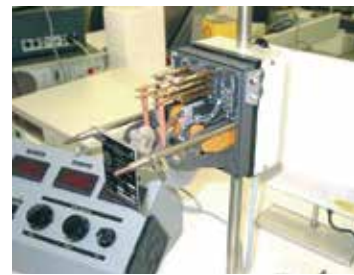
Calibration of B2 vane relay
