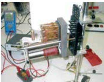
Calibration of slow pick-up and slow release B1 relay
