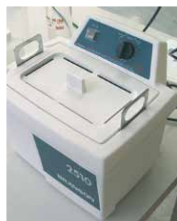
Contact cleaning Cleaning allows a better inspection of the contact and reduces the resistance.
