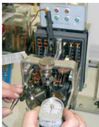
Contact pressure measurement The contact pressure is measured mechanically, evaluated and adjusted to guarantee the quality of the electrical connection.
