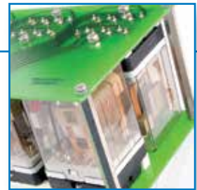
Mors Smitt D-U200 instantaneous relays plugged into PCB sockets.
