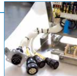
Special connectors are used for quick installation of the panel.
