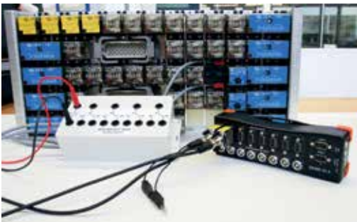
D-dock Non-intrusive commissioning and fault-finding tool.
