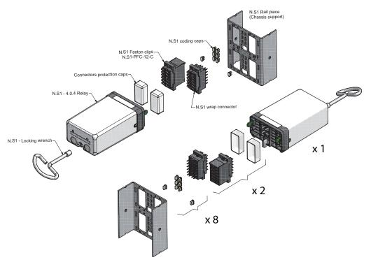
N.S1 relay are modular with automatic connector and cam locking.
