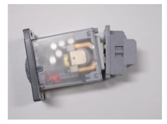
Relay partially removed from terminal block
