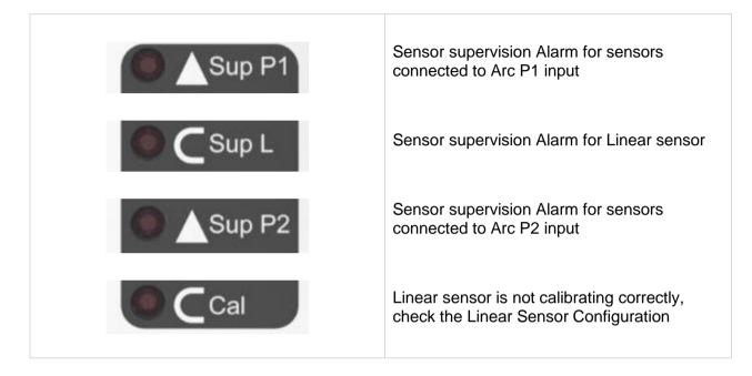
The Sensor Supervision indications will self-reset upon the alarm conditions being corrected.
