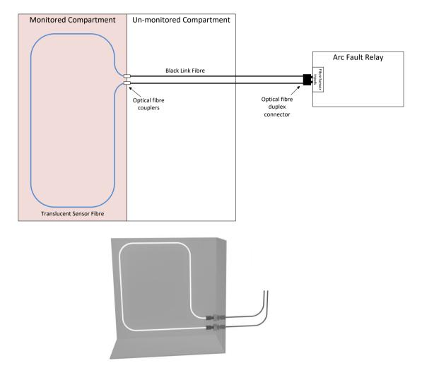
For the most effective coverage it is preferable to loop the translucent fibre within the monitored compartment or chamber as shown in the diagrams above. A light intensity of >10,000 Lux over a length of 300mm is required to cause an arc trip.
