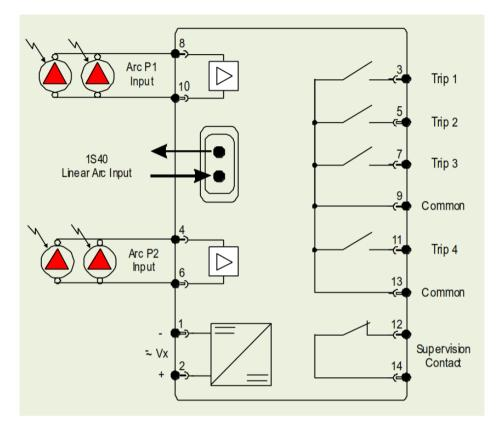
The above diagram shows the 1S27 connections (1S40 connection with 1S27 B only).
