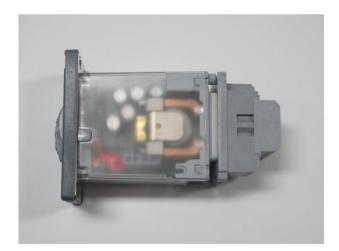
Relay plugged into a terminal block
