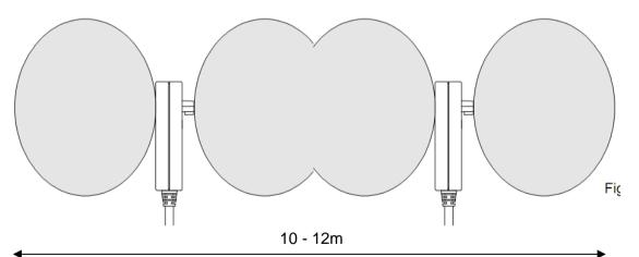
The 1S30A and 1S30B sensors may also be mixed to provide various coverage combinations, spacing's of approximately 5 - 6 m should be observed to ensure adequate detection overlap.
