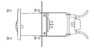
Retention of relay base when relay is removed
