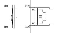
Insertion of relay and base for capturing relay base into retention plates
