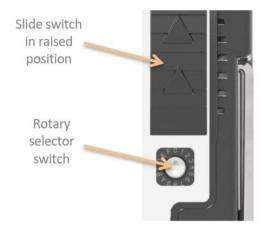
The single digit configuration code required to set the 1S27 is determined from the selection matrix shown in Table 2. The slide switch is released for the setting to be stored in memory.
