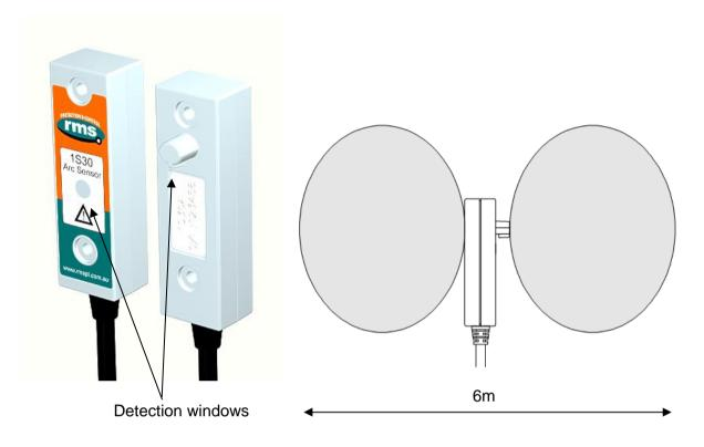
The recommended spacing for the 1S30B single detectors is approximately 5 - 6 m to ensure adequate detection overlap, this combination provides an overall coverage zone of approximately 10 - 12 m.
