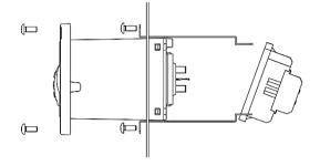
Alternative method for capturing relay base into retention plates
