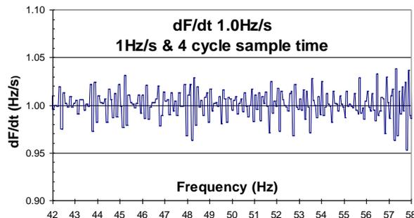
While random noise hits may cause spikes beyond the maximum error quoted these will not be of sufficient duration to cause a trip event due to the time delay setting & dF/dt rejection function.
