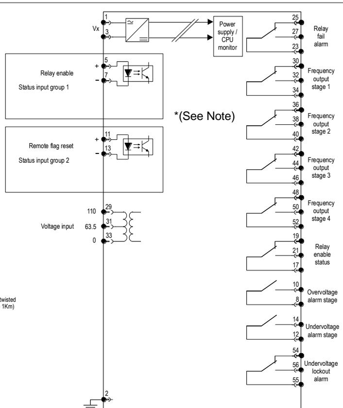
2H34 wiring diagram - Relay shown in de-energised condition
