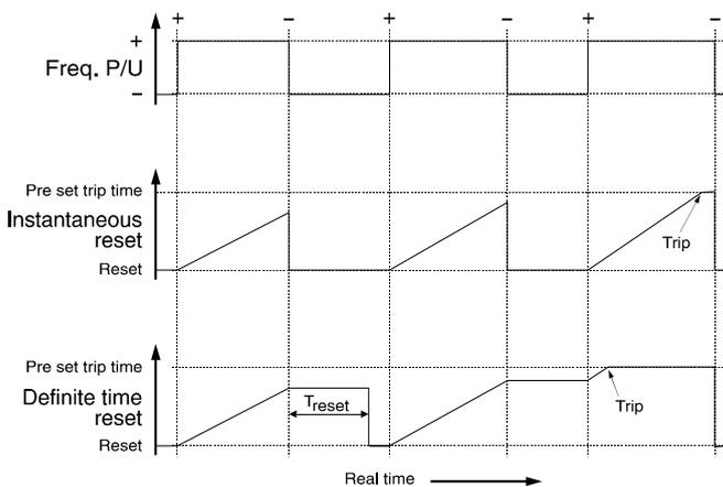
It should be noted that once the relay has timed out & the trip output initiated, the frequency element will reset instantaneously when the frequency pick up is reset irrespective of the Treset setting.
