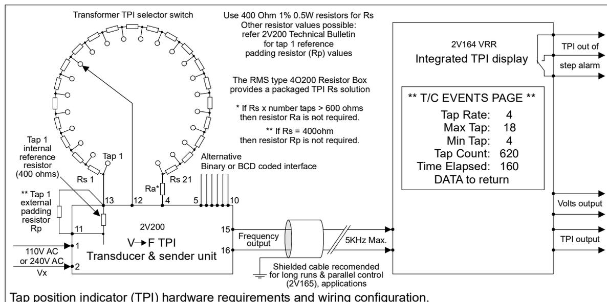
Figure 1 – Application diagram
