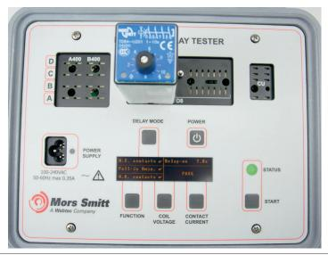
Instantaneous B400 relay failed the test: N/C contacts are not OK
