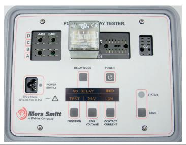
Instantaneous CU-relay passed the test
