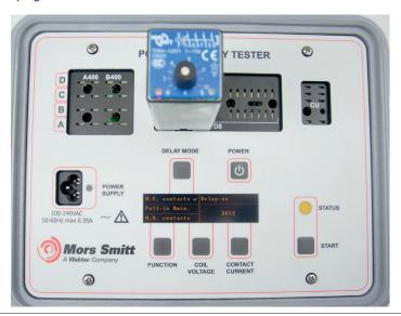
TDB4 timer relay passed the test
