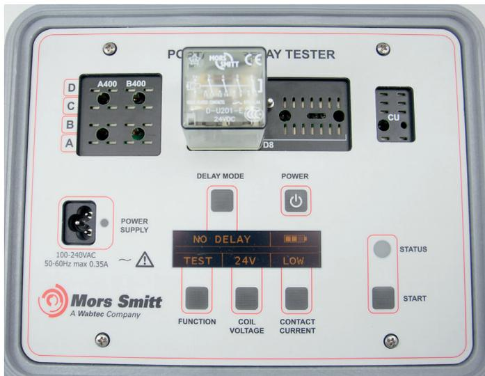
Instantaneous CU-relay passed the test
