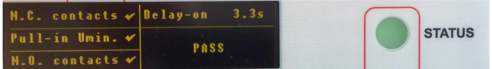
When DELAY ON or DELAY OFF is selected, the measured time delay is shown.
