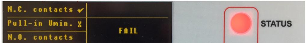
In the screen is shown with X at which test step the test failed.
