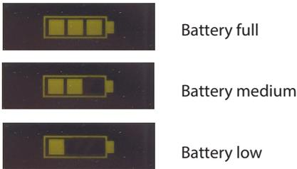
The tester will automatically switch off when not in use for approximately 1 minute. Battery lasts 8 hours (standard use). Battery charging time approximately 2 hours. During charging the tester is disabled.
