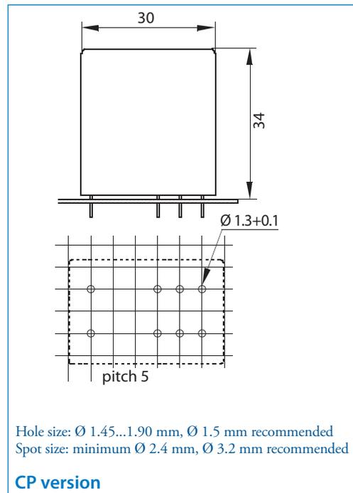
Hole size:  $\text{Ø } 1.45\text{...}1.90 \text{ mm}$ ,  $\text{Ø } 1.5 \text{ mm}$  recommended
