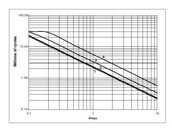
DC Current breaking capacity L/R = 20 ms; 40 ms
