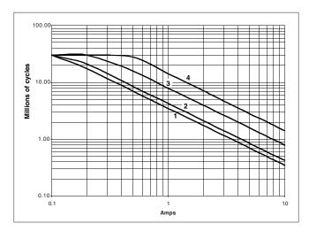
AC Current breaking capacity at  $\cos \varphi = 0.7$ ; 0.5; 0.3
