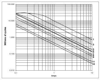
DC Current breaking capacity at L/R = 0
