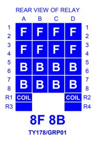
**F = Front contact**, which is made when the relay is energised. This is a normally open contact.
