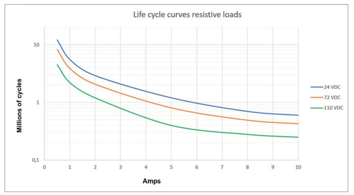
By connecting 2 contacts in series the DC current breaking capacity is increased by 50 %. Electrical lifetime is tested under laboratory conditions with switching frequency 0.33 Hz.
