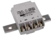
On trackside it is mounted on the rectifier output to detect an overload level on the power cell. Some versions allow detection levels adjustment by an external supply and can be calibrated for currents up to 15000 ADC. They can also incorporate a hold memory fault and a time delay to avoid tripping during charging of capacitor filters.
