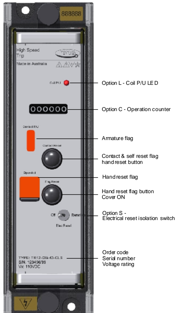
Figure 1: Front panel layout depicting flags, resets & option positions The flag and reset positions for the five contact AR5 version are set lower on the front panel.
