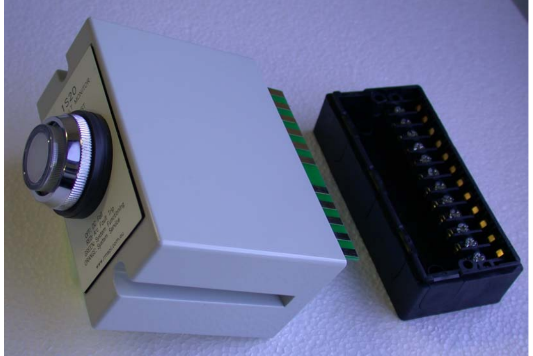
1S20 Arc Fault Monitor shown un-plugged from terminal base Note gold PCB contacts
