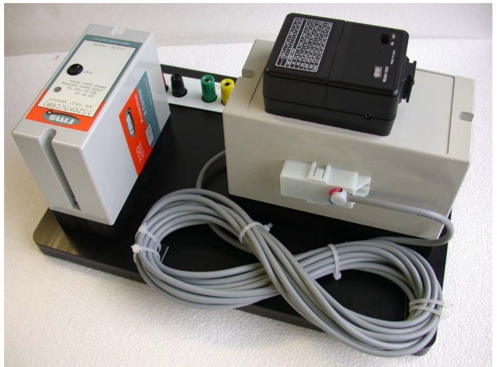
1S20 Speed of Operation Test Jig Manufactured by RMS
