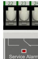
Figure 18: Self-supervision service alarm
