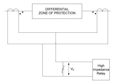
The fault current may contain a transient d.c. component current which can cause saturation of the current transformer core and thus distortion of the secondary current. Therefore in order to calculate the required setting voltage, it is assumed that one of the protection CT's saturates.
