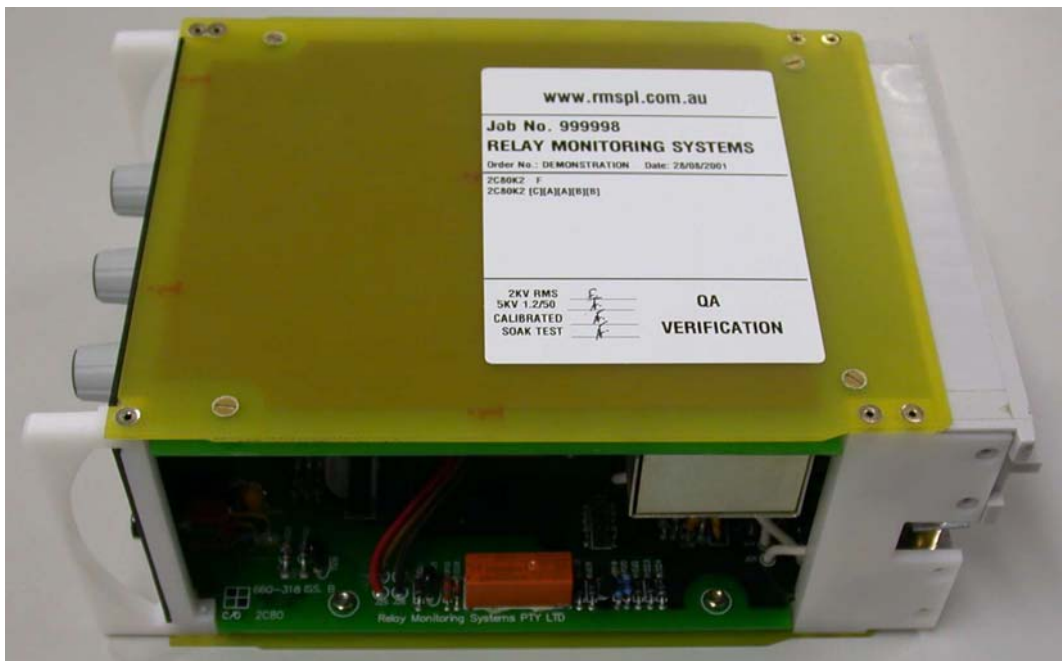
Image of generic inner relay module after removal from the outer case.
