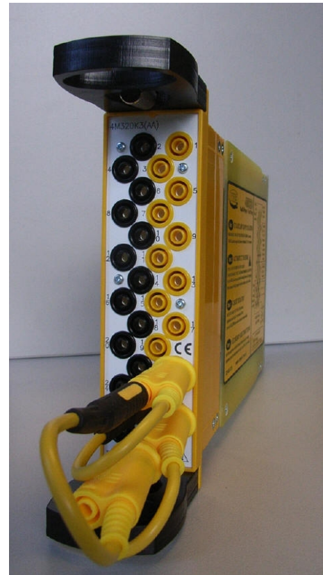
Front view showing terminals 21-23-25-27 shorted
