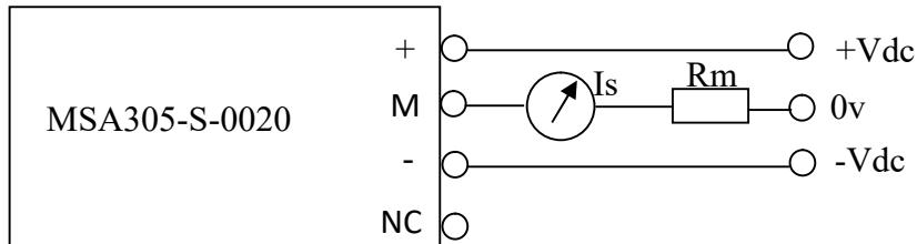
The measuring resistor  $R_m$  is determined by the user according to its application.
