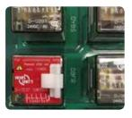
Test for voltage presence: No voltage present (LED indicator OFF)
