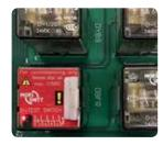
Test system by simulating energized relay: Contacts are manually switched
