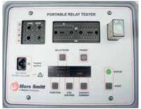
CU-relay passed the test (green LED: passed, red LED: failed)
